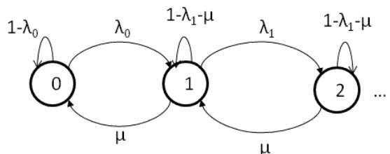
Fig. 2 The Markov Chain model of the queue
